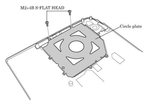
Figure 4-48 Removing the circle plate
